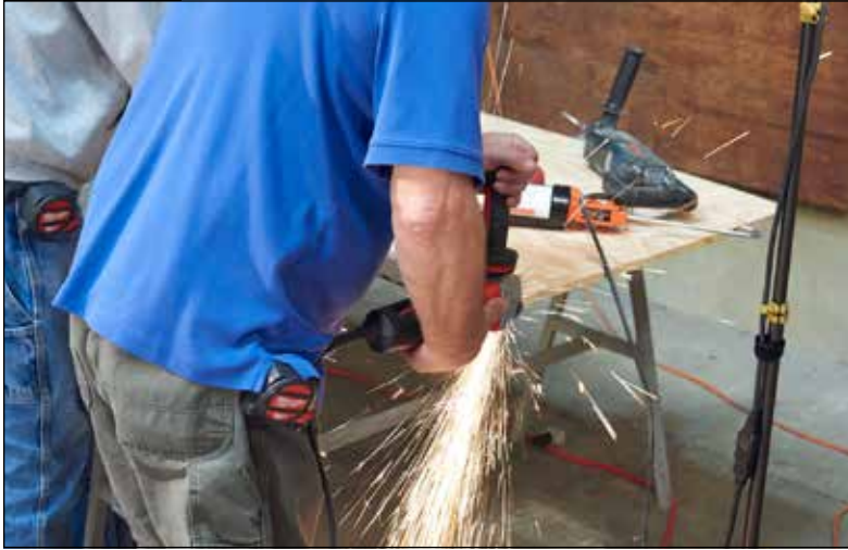
Cut 1/8" shorter to allow clearance.
