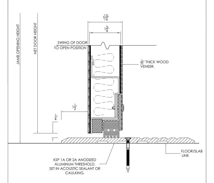
Cam Lift Door Bottom with Threshold & WDV Detail
