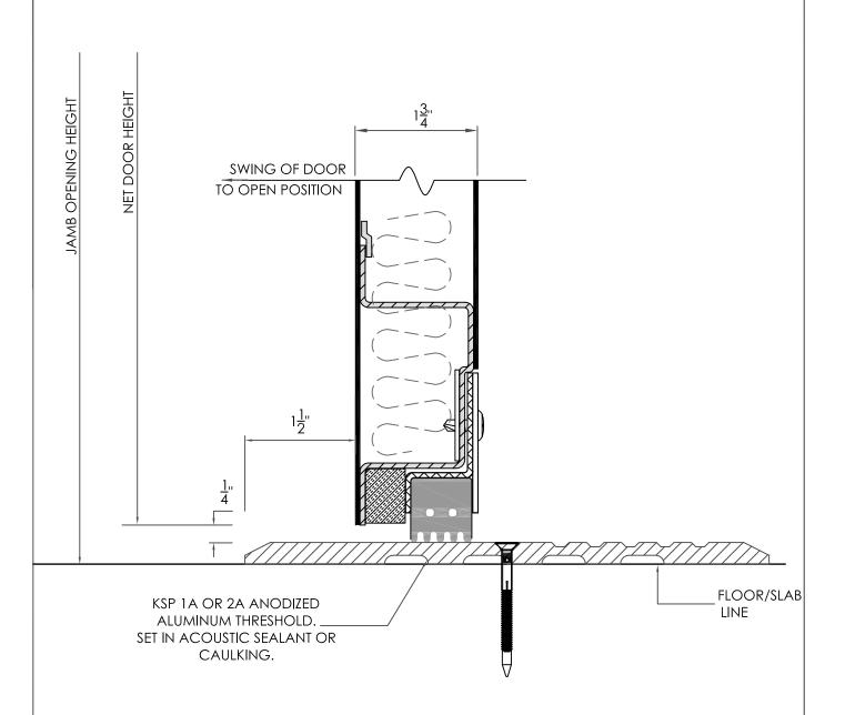
Kriegersonic Cam Lift Door Bottom with Threshold
