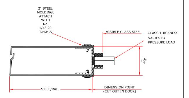
\*Laminated, fully heat tempered clear glass. Thickness and number of piles to be determined by manufacturer to suit the overpressure criteria.
