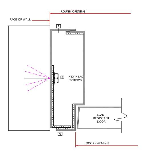
12 GA. SUB-FRAME SHIPS IN THREE (3) PIECES. 12 GA. DOOR FRAME SHIPS AS ONE WELDED UNIT.
