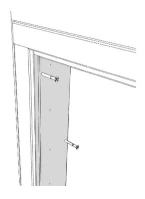
• Anchor the frame securely to the wall with anchor bolts per the size and quantity listed on the shop drawings.
