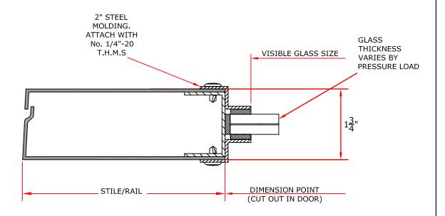
\*Laminated, fully heat tempered clear glass. Thickness and number of piles to be determined by manufacturer to suit the overpressure criteria.
